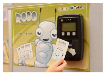
Fig. 1. Pupil touches a reader device with a contactless smart card in order to log in at the school.
