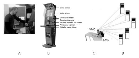
Figure 1. Use situation, service kiosk with customer's view, service clerk's VMC view with CMS and kiosk network
